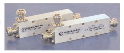
These couplers are based on Microlab CK-50N series of N type Directional Couplers Each is a multi section, quarter wave, microstrip design for indoor applications covering all wireless bands from 698 to 2,700 MHz. Units couple off a defined fraction of signal from 6 to 30 dB with minimal reflections or loss.
